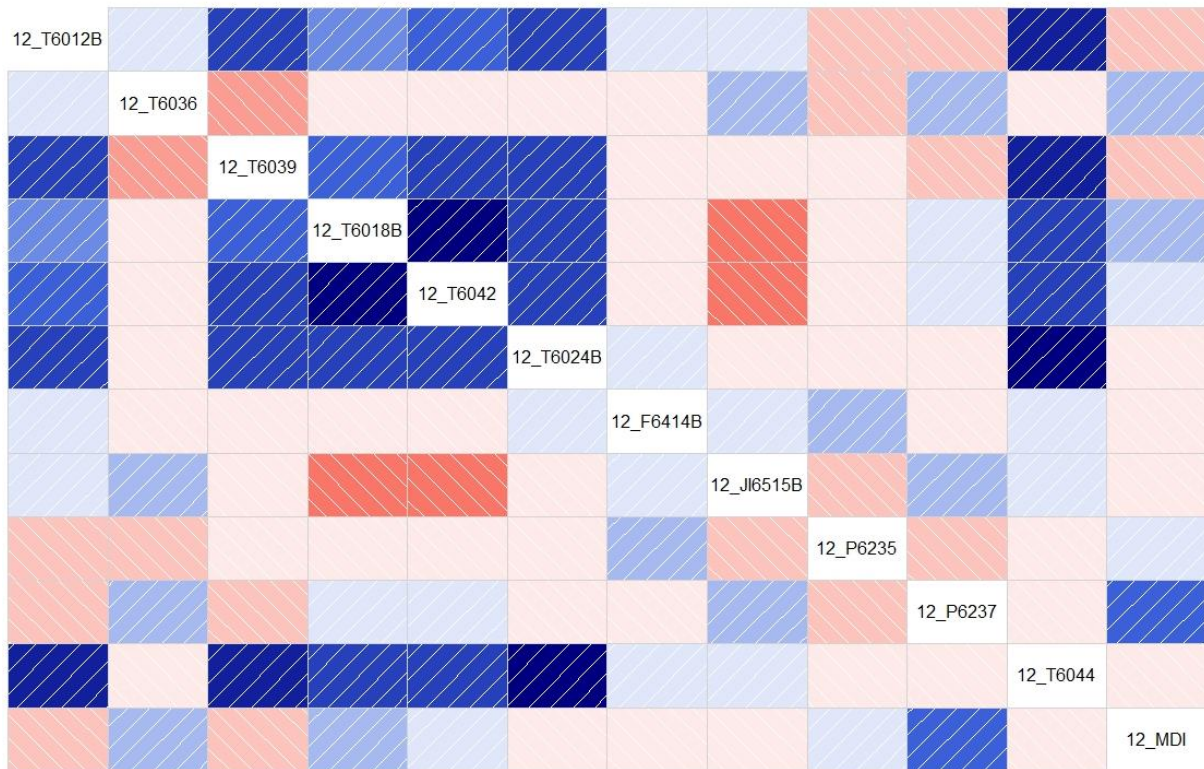
Figure 4. 10 - Correlogram for Huntsman single compressor data. Color blue denoted positive correlation and red denotes negative correlation. The intensity of the colors is an indication of the value, with higher values of correlation having more intense colors.
