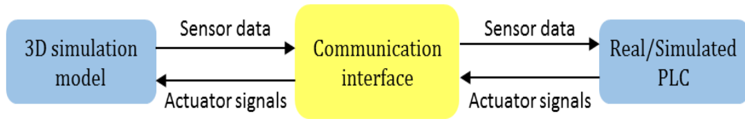
Figure 3.3: Exchange of data between simulation model and external PLC
